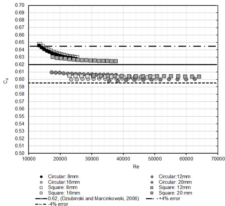
Figure 1. Calibration results for circular and square orifices
